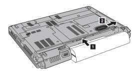
6. Slide the battery latch 1 to the locked position 2.
